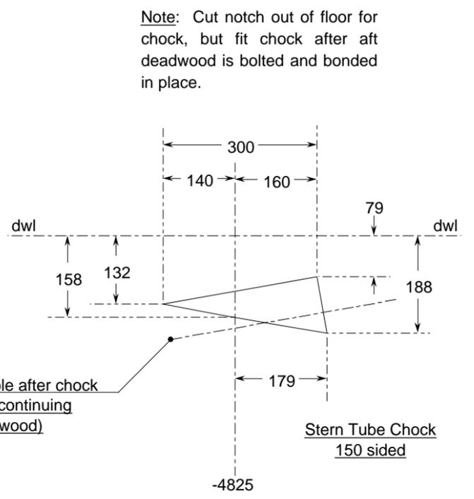
Note: Aft deadwood bolts are on centreline. Bolts, nuts & washers are stainless steel Grade 316 S16 & A4
