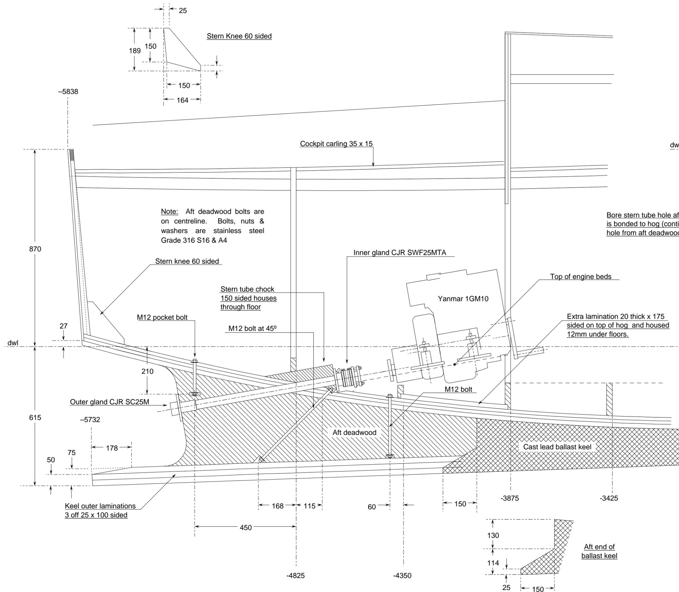
Note: Cut notch out of floor for chock, but fit chock after aft deadwood is bolted and bonded in place.
