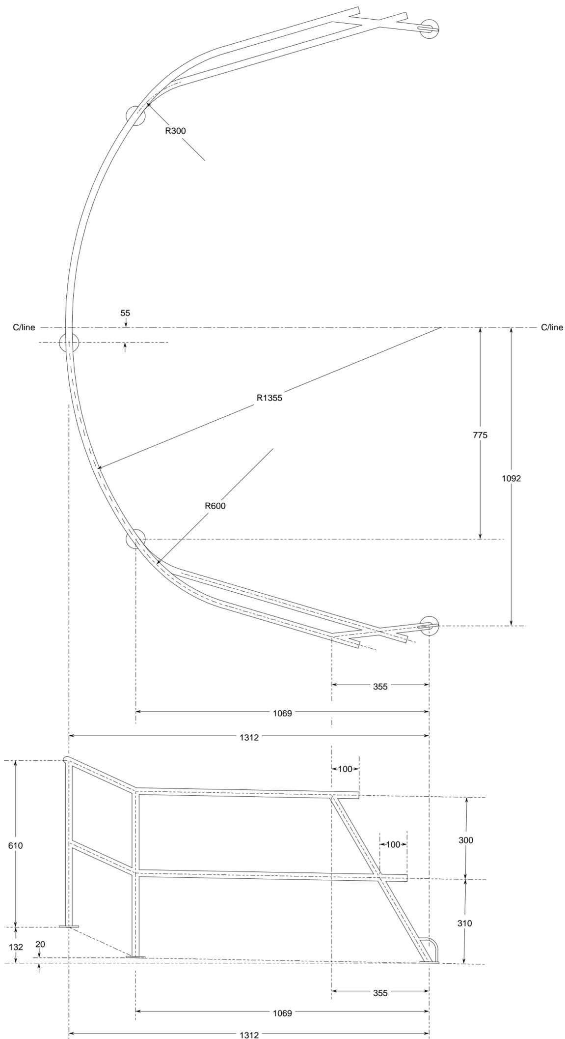
**Note:** Stern pulpit is made from  $\varnothing 25 \times 1.5$ mm wall S/steel tube, polished after fabrication.
