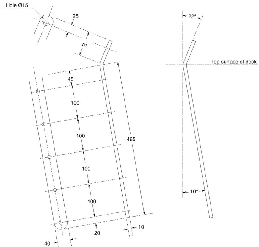
**Note:** Backstay plate made from Stainless Steel Grade 316, polished after fabrication. Plate made from a single piece, min radius of bend 20mm.
