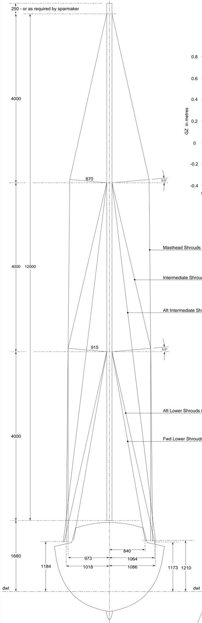
All shrouds and stays are 7mm 1 x 19 stainless steel wire rope terminating in swageless eye (or fork) terminals at the top and open body swageless/body/integraltoggle bronze rigging screws at the bottom, size 1/2" UNF.
