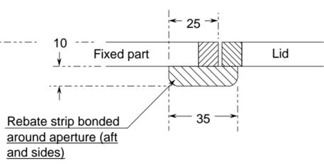
Note: Lid hinged on 3 off dovetail hinges let flush into top.
