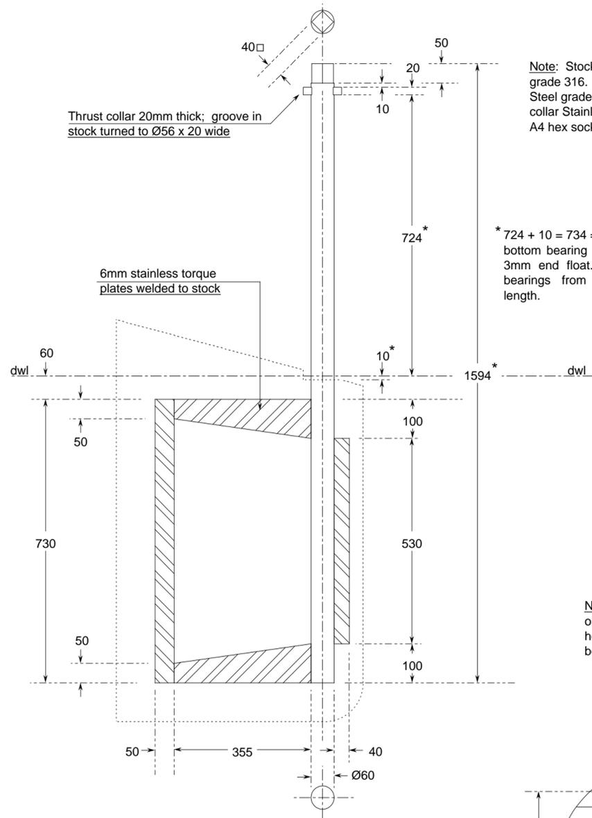
Note: Stock Ø60mm true bar Stainless Steel grade 316. Torque plates 6mm Stainless Steel grade 316 welded to stock. Thrust collar Stainless Steel grade 316 with grade A4 hex socket screws.
